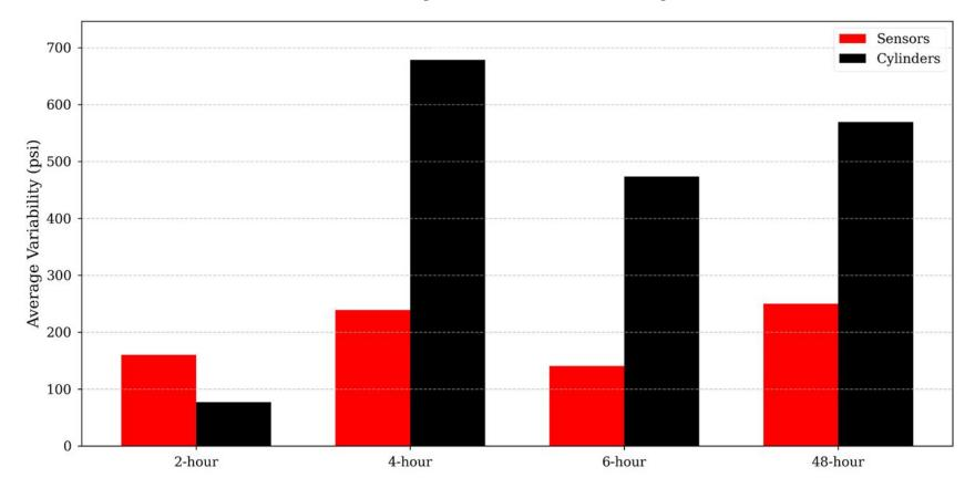
• The sensors had significantly less variability than the cylinders at 4, 6, and 48-hours
