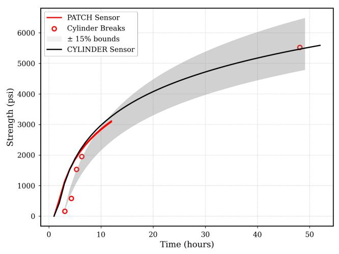
• The sensor in the patch was unplugged after 10 hours for traffic opening
