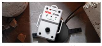
In response, the team conducted extensive research into concrete's resonant characteristics while curing, culminating in the discovery of the REBEL® concrete sensor. This groundbreaking technology can reliably and rapidly assess the strength of concrete as it cures to help DoTs open
